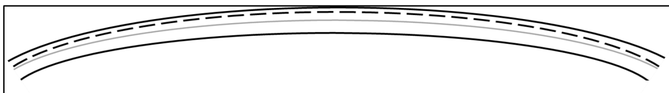
Figure 2.1: Path deviation in transfer tube: the actual source path (---) deviates from the ideal source path (—).
