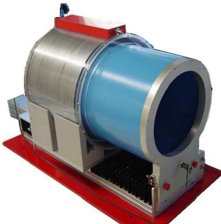
Figure 12: The GROVEX extrapolation chamber maintained at PTB
